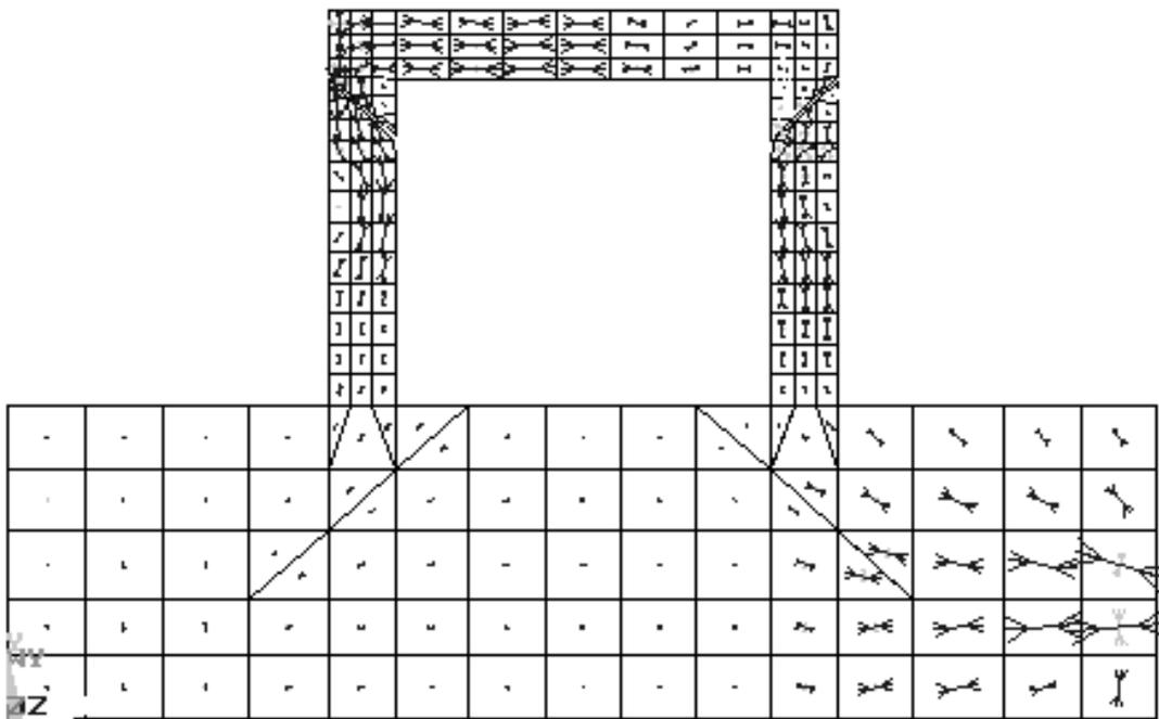
Figure 3b. Principal stresses by TDA at  $50\mu\text{sec}$ .
